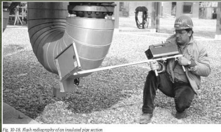
Fig. 10-18. Flash radiography of an insulated pipe section
